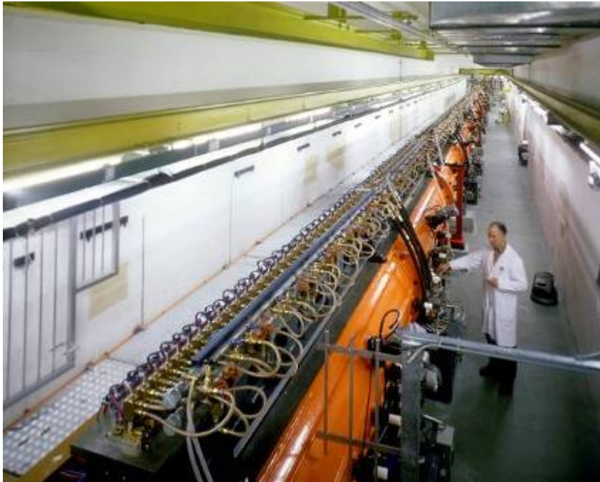
CERN Linac2 Drift Tube Linac accelerating tank 1 (200 MHz). The tank is 7m long (diameter 1m) and provides an energy gain of 10 MeV.
